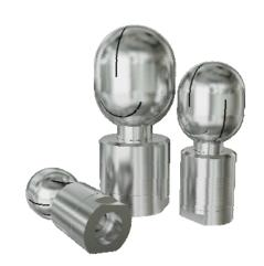
Series SB rotary spray ball is a self rotating tank cleaning device. The spray ball is driven by the cleaning fluid. The ball has knife through cuts on its surface, which allow the fluid to pass through it and create powerful jets. Powerful spray jets cover cleaning of tanks all around 360°.
